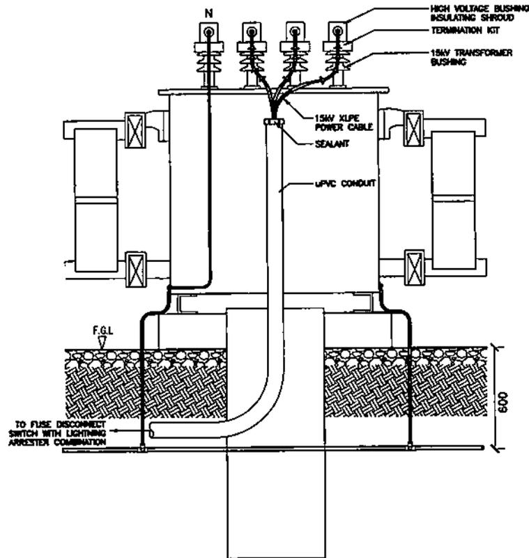
**TRANSFORMER HIGH VOLTAGE CABLE TERMINATION**
